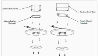
Typical Installation Views mounting directly into standard octagonal or square junction Box (left).
