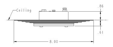
UPC: 692193787907: Diffuser, 120VACin, 2700k, 14.9Watts, 1440.7 Delivered Lumens, 96.7 Lm/W (measured) Mfr Item Code: S085C01LP327DM115w
