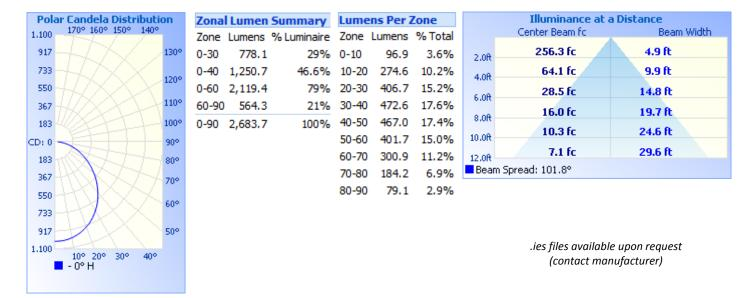
M1011LP30: Diffuser, 120VACin, 5000k, 29.0 Watts, 2683.7 Delivered Lumens, 92.5 Lm/W (measured)
