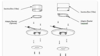
Typical Installation Views mounting directly into standard octagonal or square junction Box.
