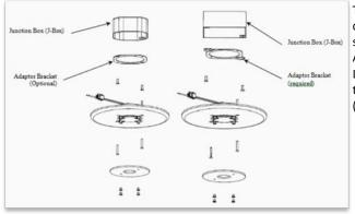
Typical Installation Views mounting directly into standard octagonal or square junction Box (left).
