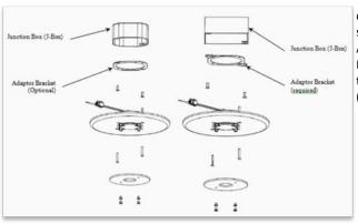
Typical Installation Views mounting directly into standard octagonal or square junction Box (left).
